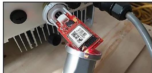
**STEP 4:** The circuitry has a small SMD button at the bottom of the antenna as shown.
